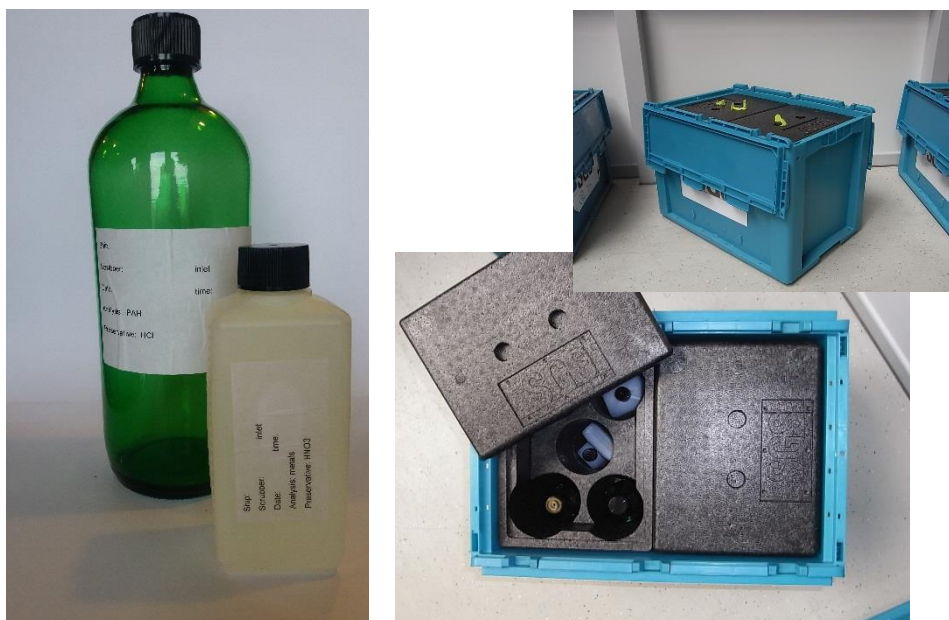
Figure 1: sample bottles for PAH and metals analysis with cooler box for transport used in Programme 1
